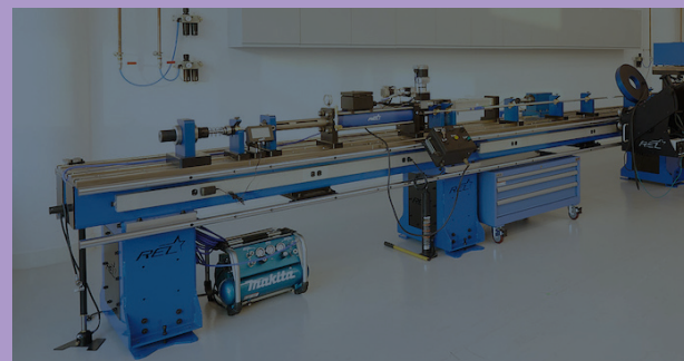
Split Hopkinson Pressure Bar Up 10000/s strain rate High speed DIC Up to 250°C Direct impact capability
